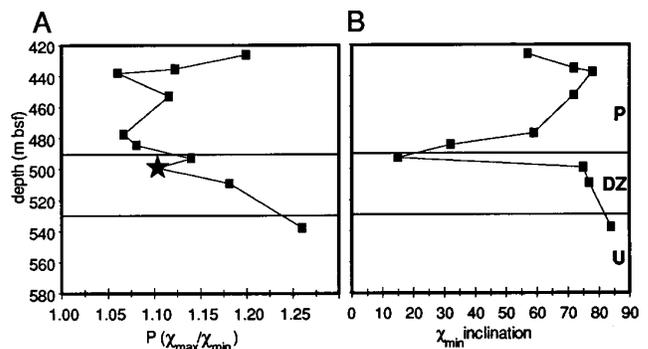
Figure 5. A: Degree of anisotropy vs. depth (as in Fig. 4) for anisotropy of high-field-susceptibility results from Site 948. Star indicates sample from scaly fabric interval near top of decollement. B: Inclination of minimum high-field-susceptibility axes for Site 948 (as in Fig. 2).
