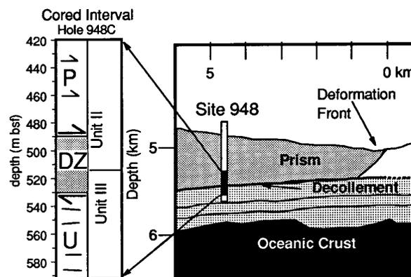
Figure 1. Diagram of Barbados accretionary prism, illustrating major tectonic features and location of ODP Site 948. Enlargement at left shows cored interval of Hole 948C (420–590 m bsf). This interval is subdivided into three structural domains: P is accretionary prism (420–490 m bsf), DZ is decollement zone (490–530 m bsf), and U is underthrust sediment (>530 m bsf). Half arrows indicate thrust faults.
