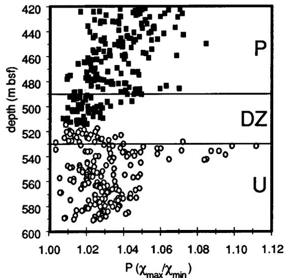
Figure 4. Degree of anisotropy vs. depth for Site 948. Solid squares indicate results from lithological unit II; circles indicate results from lithological unit III.
